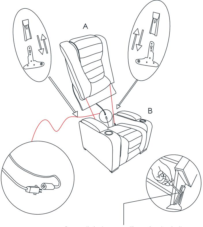
To remove the back, use a screwdriver pressing outward on the back tab in the receiver on both sides and lift the back from the base
