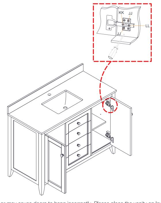
Uneven floor may cause doors to hang incorrectly. Please place the vanity on level surface, or adjust the levelers at the bottom to ensure that it is perfectly level. If necessary, doors can be adjusted with a Philips screwdriver at the adjustable hinges.
