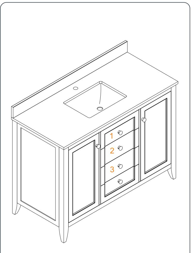
In case drawers need to be removed, each drawer is individually numbered underneath the drawer box with the corresponding number on top of the dust partition, inside the case.
