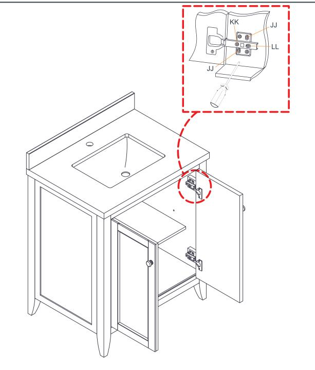
Uneven floor may cause doors to hang incorrectly. Please place the vanity on level surface, or adjust the levelers at the bottom to ensure that it is perfectly level. If necessary, doors can be adjusted with a Philips screwdriver at the adjustable hinges.
