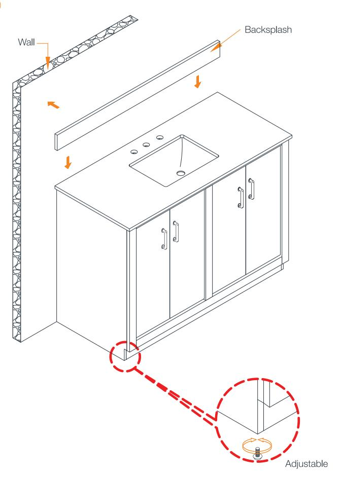
For application of backsplash (B) to drywall: Make sure the wall is smooth and flat. Clean the wall and the back of the backsplash (B) with damp cloth to remove any grease or debris. Apply thin-set adhesive, and then set the backsplash (B).
