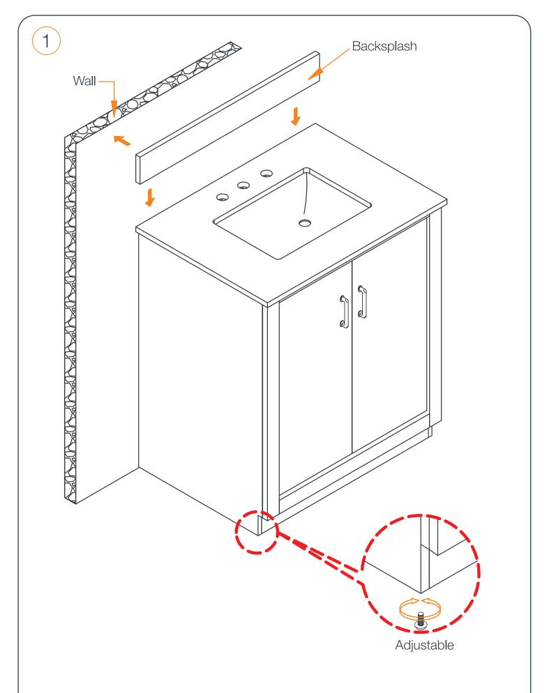
For application of backsplash (B) to drywall: Make sure the wall is smooth and flat. Clean the wall and the back of the backsplash (B) with damp cloth to remove any grease or debris. Apply thin-set adhesive, and then set the backsplash (B).
