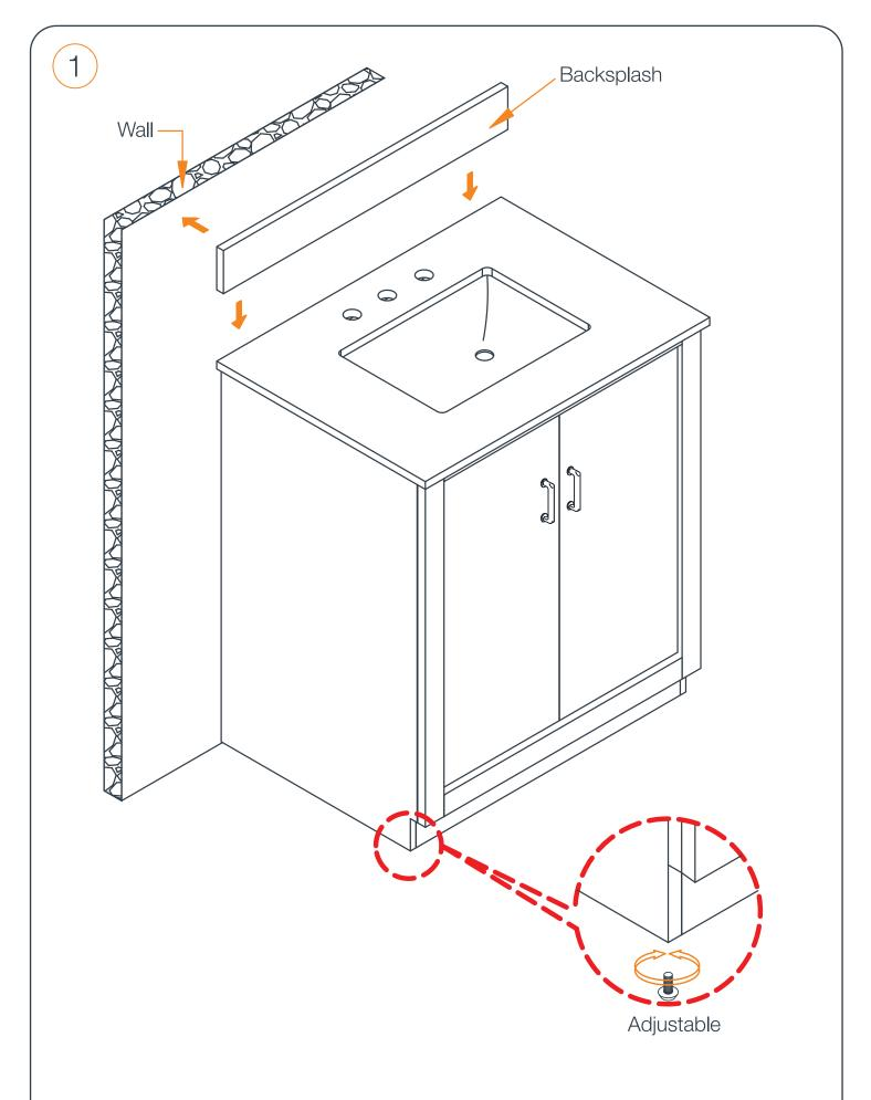
For application of backsplash (B) to drywall: Make sure the wall is smooth and flat. Clean the wall and the back of the backsplash (B) with damp cloth to remove any grease or debris. Apply thin-set adhesive, and then set the backsplash (B).
