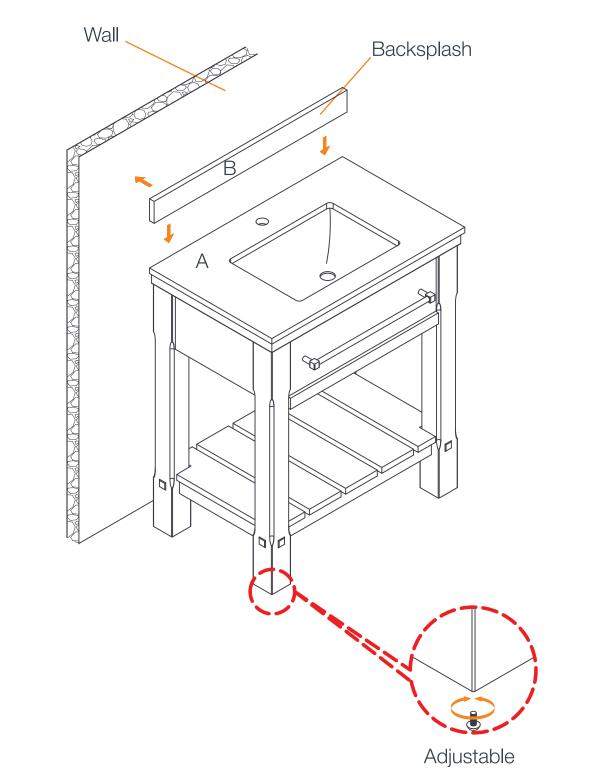
For application of backsplash (B) to drywall: Make sure the wall is smooth and flat. Clean the wall and the back of the backsplash (B) with damp cloth to remove any grease or debris. Apply thin-set adhesive, and then set the backsplash (B).
