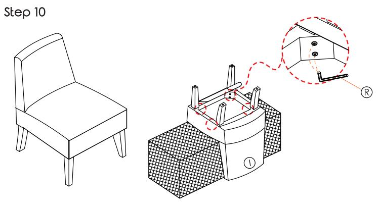
Make sure the chair feet are level, then fully tighten all the bolts at this step;
