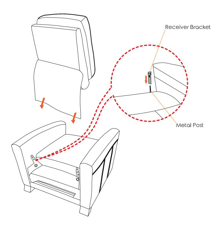
To remove the back, use a slotted screwdriver pressing outward on the back tab in the receiver on both sides and lift the back from the base
